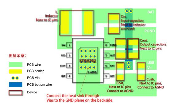
Please have C<sub>IN.</sub> C<sub>OUT</sub>, and L placed just next to the IC pins so that the power traces are kept to the shortest to achieve a good performance of ETA9742 and good EMI.
